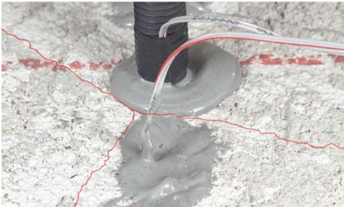
FIGURE 13 Concrete cracking during the application of load/unload cycles Source: Own elaboration.
