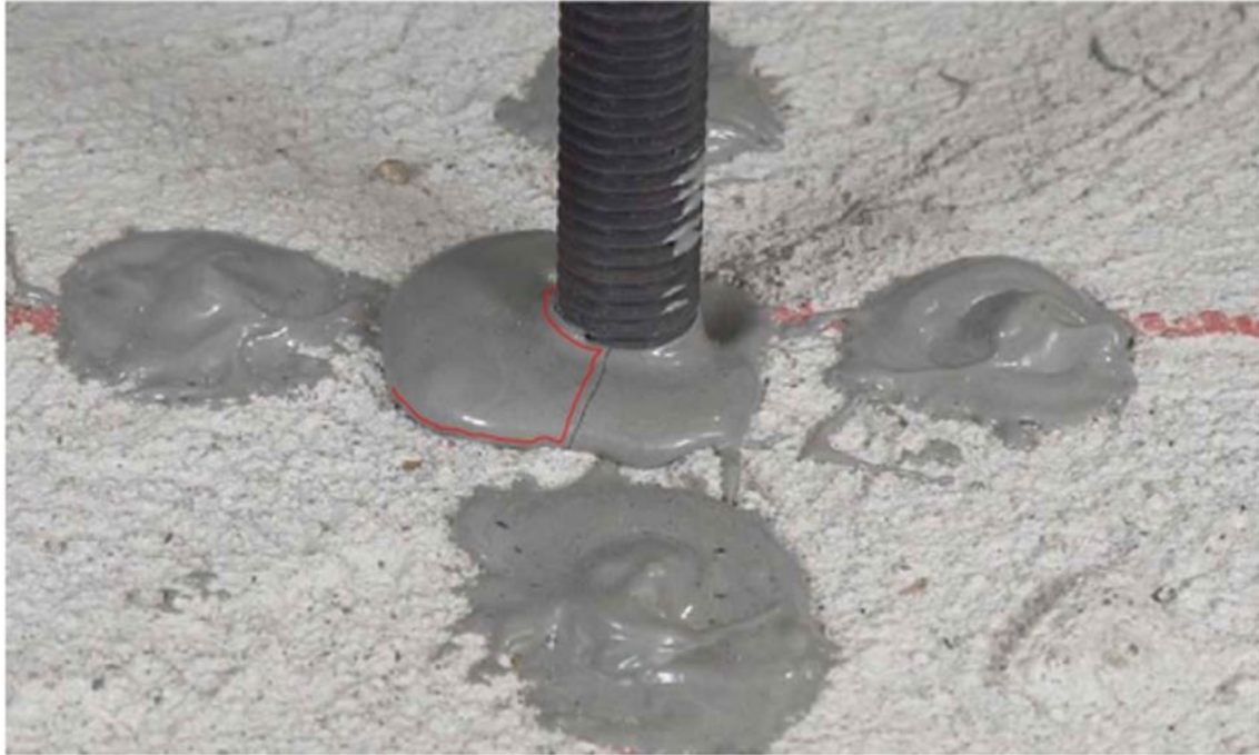
FIGURE 14 Epoxy adhesive cracks during loading and unloading cycles Source: Own elaboration.
