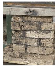
FIGURE 11 Failure of the masonry wallette under the compression test
