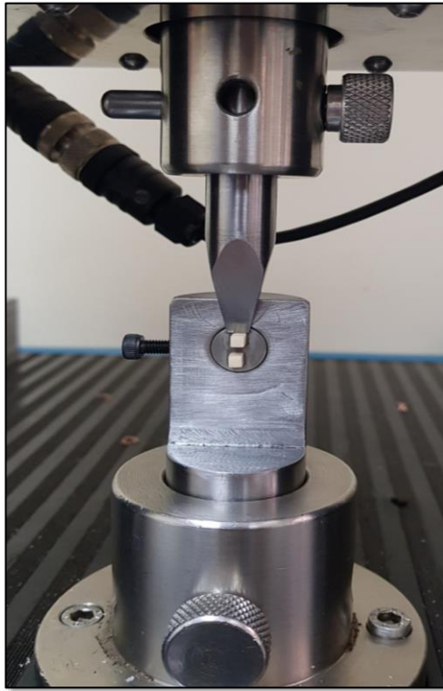
FIGURE 2 Shear Bond Strength Test Source: the authors.
