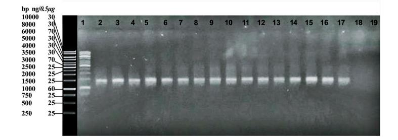
**Figure S6.:** Verification of the amplification of the 16S rRNA. A 1 % agarose gel was run in 1X TBE buffer at 80 V for 1 hour and 30 minutes, treated with the Ez Vision intercalant (AMRESCO, USA) and photodocumented in the Smart Doc Imaging Enclosure Benchmark Accuris E300 UV at a wavelength of 302 nm. In lane 1, the molecular marker 1 kb (Promega, USA) is observed; lanes 2 to 16 were loaded with *E. coli* isolates 1 to 17, respectively; and lane 18 is the negative control.
